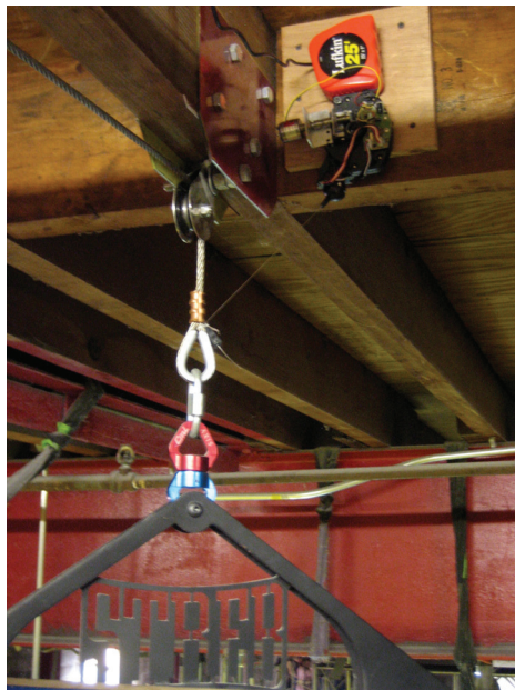
Figure 5. Extended-range Pendaphone hardware attached above the performance wall. The line from the Pendaphone connects to the rigging used by the performers to ascend the wall. The larger retraction spring in the tape measure replaces the smaller original spring in the Gametrak, allowing the Pendaphone to track 3D motion from floor to ceiling. © 2009 Byron Lahey.
