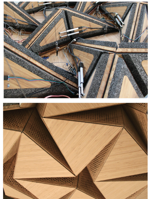
Figure 6. (above) Variable surface configuration through folding properties; (below left) circuit diagram and wiring network; (below right) wiring of prototype surface with actuators from above, and folded surface from below. © 2012 RVTR.
