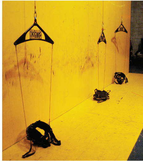
Figure 6. Custom harnesses that allow for free rotation about the torso and rigging line axes. These harnesses, similar to those used for special effects stunt-work, allow the performers to flip, twist, and move freely across the wall. © 2009 Elizabeth Streb. Photo © 2009 Byron Lahey.
